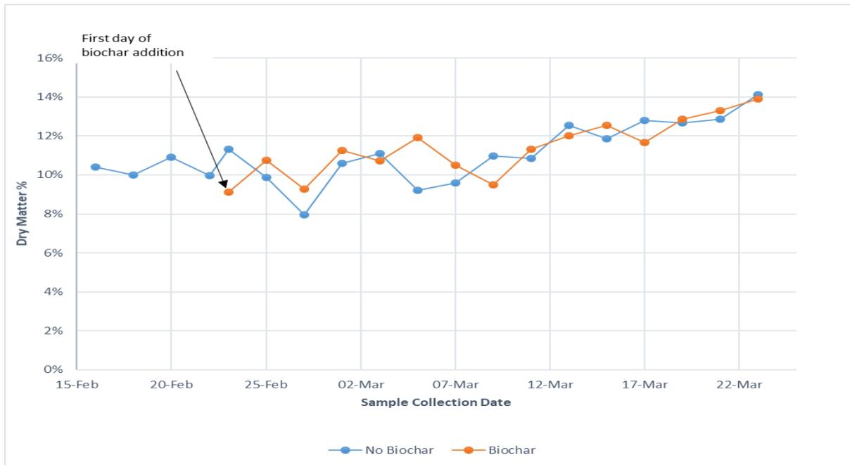
Figure 4. Dry Matter Content of Manure after Biochar Addition
