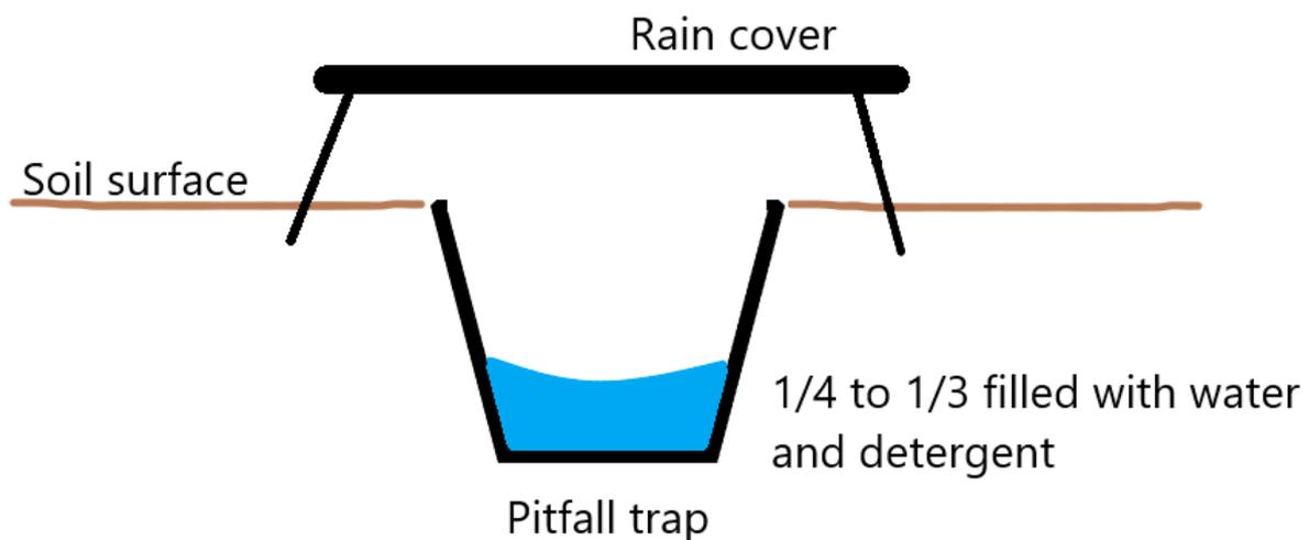
Figure 2. Pitfall trap set up. Showing trap edge flush with ground surface, rain cover plus supports and the water fill level.
