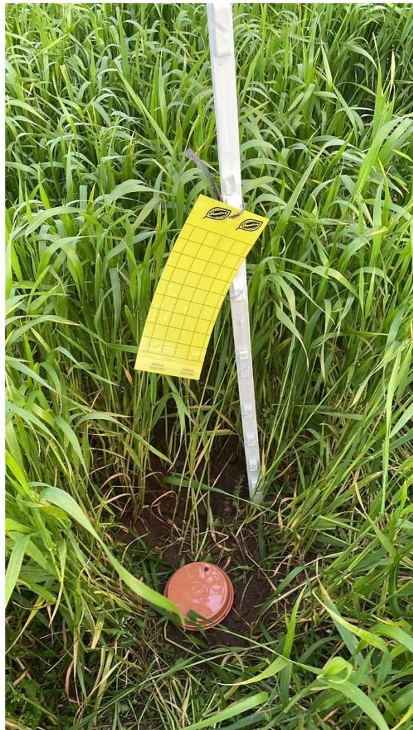
Figure 4. Pitfall trap and sticky trap in situ.
